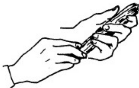
Fig. 1 The three sections of a cigar, filler, binder and wrapper, are put together first by gathering the filler leaves and compressing them evenly in the shape of a cigar.
