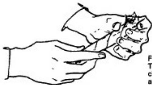
Fig. 5 The bunch is then placed on the wrapper and the operator encloses it, rolling the wrapper on spirally.
